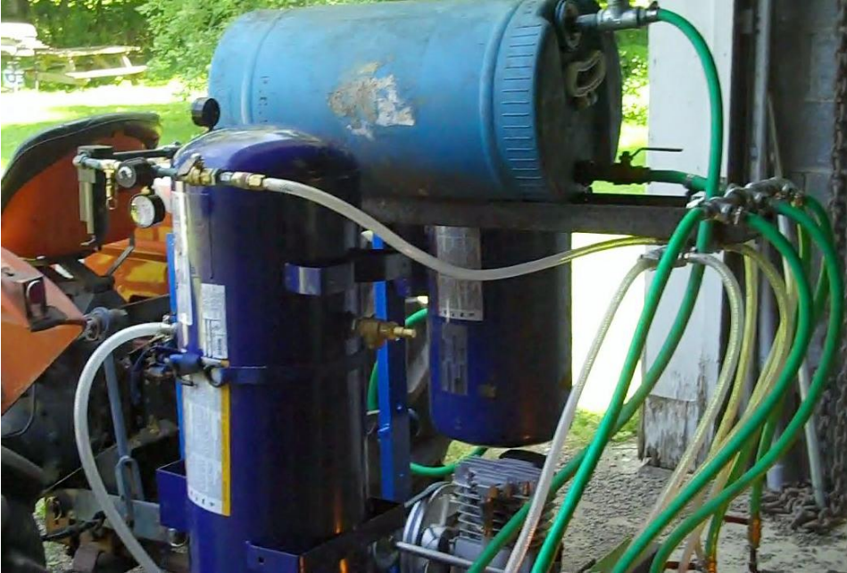
Dolan redesigned his flame weeder to run efficiently on waste vegetable oil.
