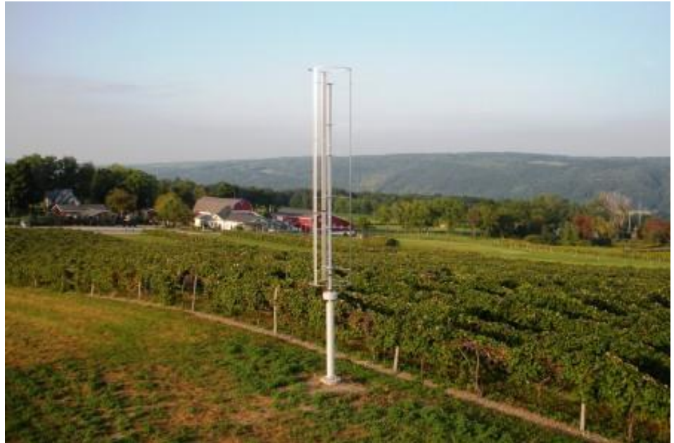
The turbine will generate up to 1.2 kW of electricity, about 2000 kW hours per year
